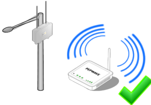
Figure 4 – Orienting the antenna vertically allows signals to span out.
